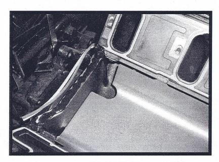
Install intake manifold assembly carefully on engine. Do not smear silicone, if smeared, remove and reapply.
