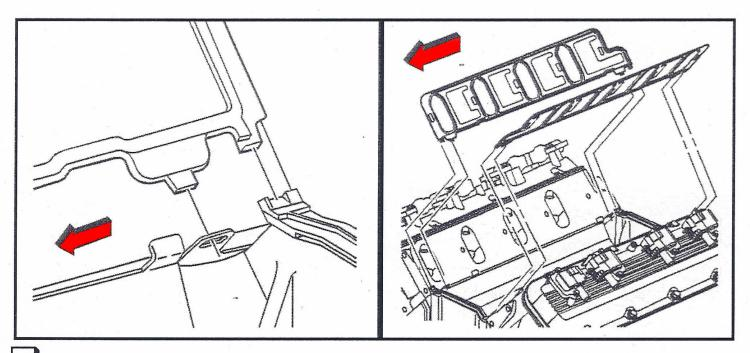
Apply a thick bead of black RTV silicone on the center valleys of the block, front and back. Run the bead all the way to the gasket edge.
